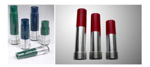
Long venture style nozzles yield about a 40% greater production rate than straight boron nozzles. The internally tapered design of the venture nozzle accelerates and evenly distributes the a brasive over the entire blast pattern. These nozzles are designed for use with a 1-1/4" I.D. blast for maximum cutting on hard-to-clean surface.
